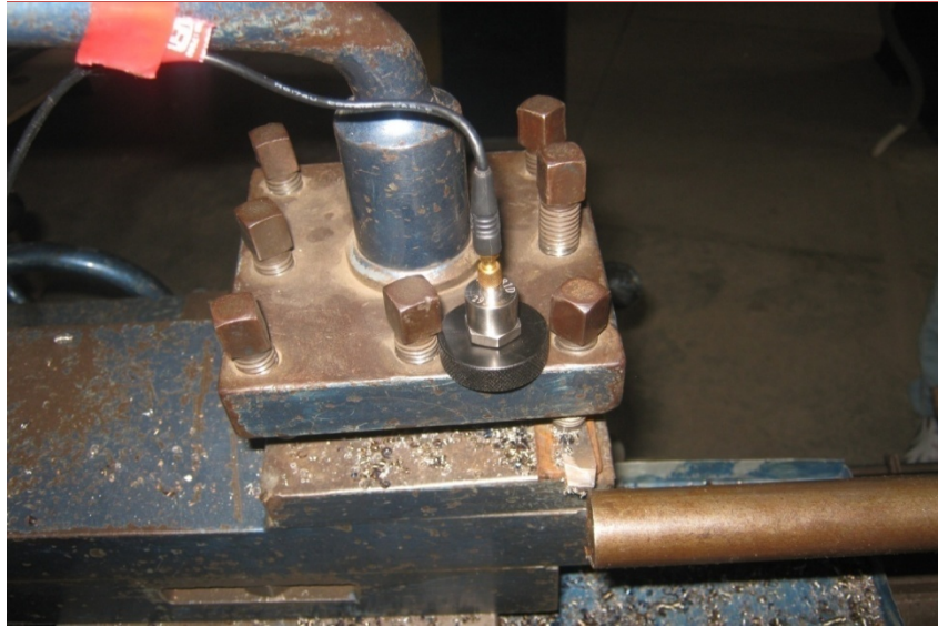
Figure 3.1: Vibration sensor mounted on tool post
