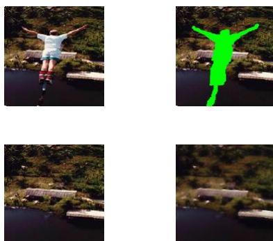
Figure 3 (a) (Extension) Original image (b) mask of input image (c) after inpainting (d) after Bregman iteration Algorithm
