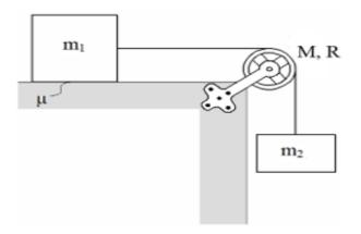
The pulley mass-system starts moving from rest. The rope does not slip over the pulley during the motion
