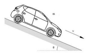
A car with mass *m* and velocity *v* is traveling down the road with a slope angle  $\theta$ . The car suddenly applies brakes with a constant force off.
