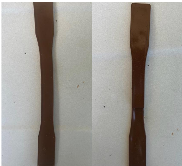
Figure 8: Images of Biocomposite Samples Before and After Tensile Test
