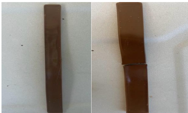
Figure 10: Images of Biocomposite Samples Before and After 3 Point Bending Test
