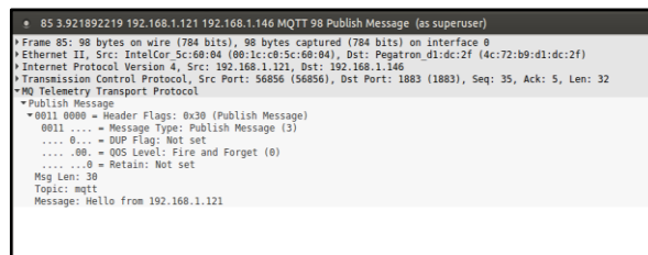
Figure1: Tracing messages using WireShark-I
