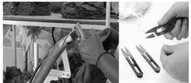
**Fig 5: Manual vs Automatic thread trimming**
