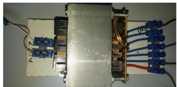
Figure 3. Primary and secondary connections of transformer with 1 input and 6 outputs with 90 VA power
