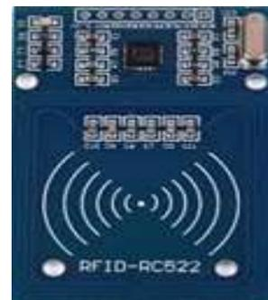
**D. RFID Tags:** RFID tags are passive tags which contain unique number. Whenever a passive tag comes in range of RFID scanner it send this unique number to the RFIDscanner. **Passive** tags wait for a signal from an **RFID**reader. The reader sends energy to an antenna which converts that energy into an RF wave that is sent into the read zone. Once the tag is read within the read zone, the **RFID** tag's
