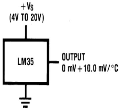
**Figure 1.** Basic Centigrade Temperature Sensor
