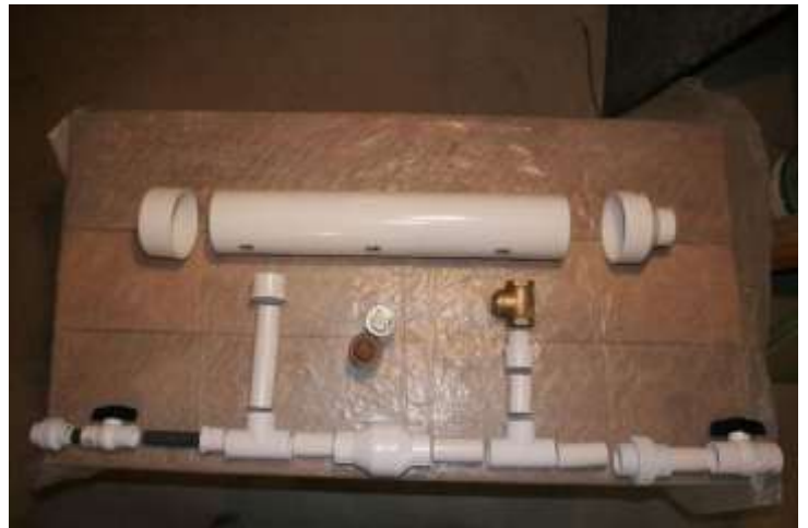
Fig 2. Disassembled Automatic Water Pump
