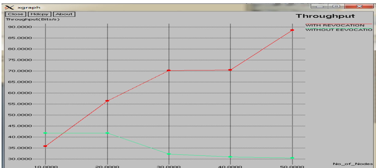
Fig 9: Throughput Vs Number of Nodes
