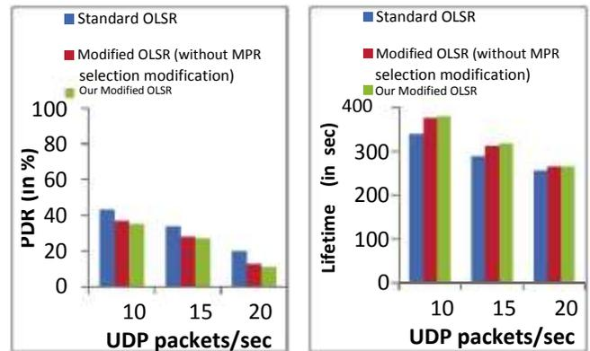
(a)PDR for various traffic rate (b)Network Lifetime for various traffic rate
