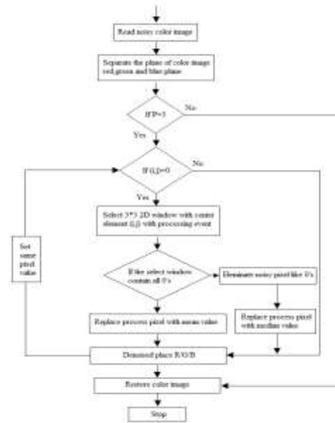
Fig.3.1 Flowchart- Proposed Novel Algorithm based for color images.
