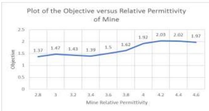
**Figure 4:** Plot of the objective with changing mine relative permittivity (soil-mine contrast)
