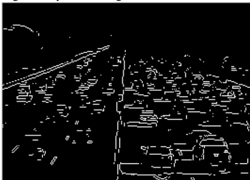
Fig 4: Edge detection using Prewitt Filter
