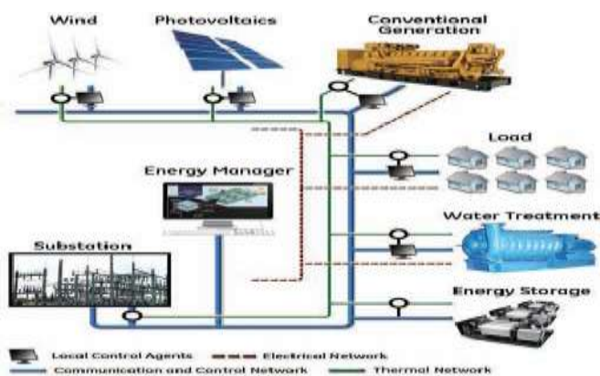
Figure 1: Microgrid power system
