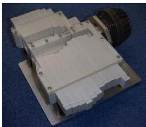
**Figure 3:** Artificial model of the human vocal tract by Umeda and Teranishi [18].
