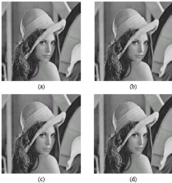
Fig. 5. Original and watermarked gray-scale Lena images (a) original, (b) 44.87 dB with 0.30 bpp, (c) 37.82 dB with 0.65 bpp, and (d) 32.92 dB with 1.00 bpp.
