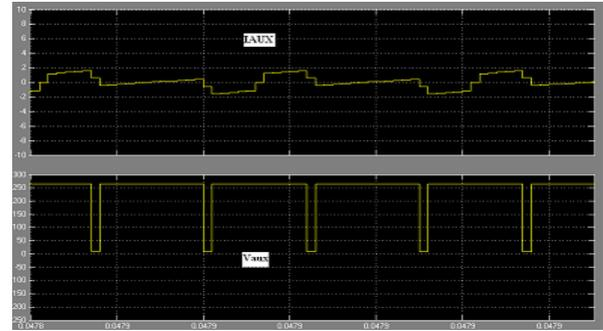
Fig. 6. Key waveforms of the converter for  $D > 0.5$ .
