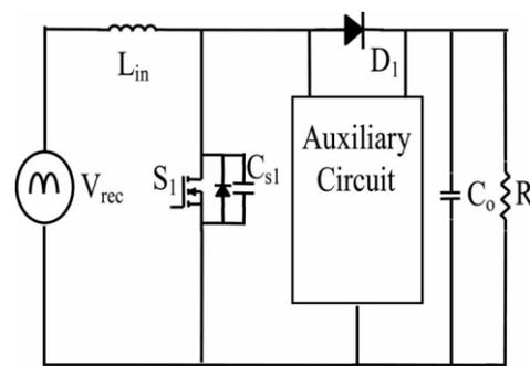
Fig. 3. Placement of ZVS auxiliary circuit in boost PFC converter.
