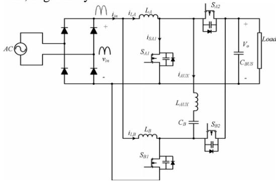
Fig. 5. Proposed ZVS interleaved boost PFC schematic.
