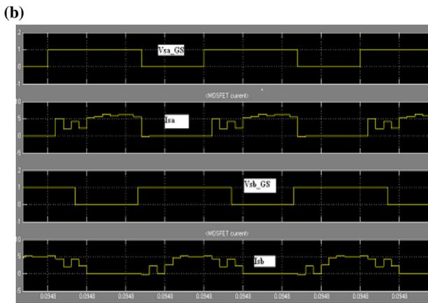
Fig. 12 Simulation waveforms of the main switches  $S_a$  and  $S_b$  ( $D > 50\%$  and load current 1.5A). (a) ZVS. (b) ZCS
