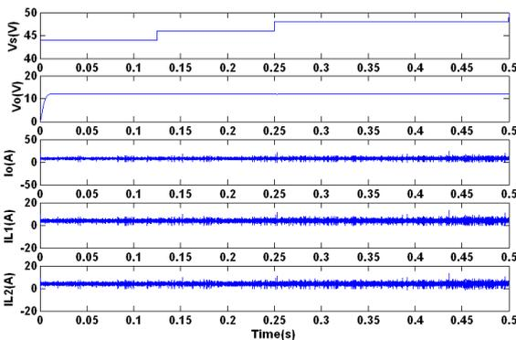
Fig. 16. Simulation results for ZCS Interleaved Buck Converter ( $V_{sInput}$  Voltage,  $V_o$ -Output Voltage,  $I_o$ -Load Current,  $I_{L1}$  and  $I_{L2}$ -Inductor Currents)
