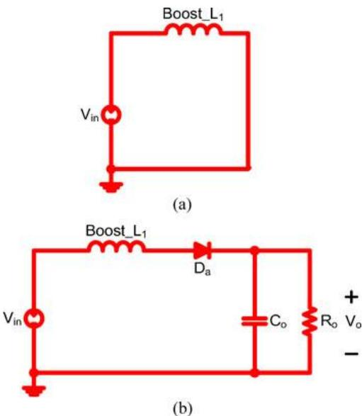
Fig. 6 Equivalent circuits for the boost inductor ( $D < 50\%$ ). (a) Boost\_L<sub>1</sub> in the stage [t<sub>b</sub>-t<sub>c</sub>], stage [t<sub>d</sub>-t<sub>e</sub>], stage [t<sub>e</sub>-t<sub>f</sub>], stage [t<sub>f</sub>-t<sub>g</sub>] and stage [t<sub>h</sub>-t<sub>i</sub>]. (b) Boost\_L<sub>1</sub> in the stage [t<sub>a</sub>-t<sub>b</sub>], stage [t<sub>c</sub>-t<sub>d</sub>] and stage [t<sub>g</sub>-t<sub>h</sub>].
