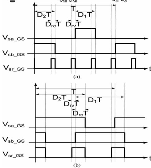
Fig. 2 Switching waveforms of the main switches  $S_a$  and  $S_b$  and auxiliary switch  $S_r$ . (a)  $D < 50\%$  mode. (b)  $D > 50\%$  mode.
