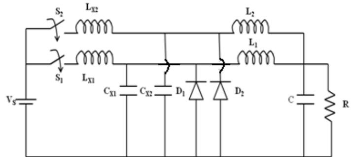
Fig:14-schematic diagram of ZCS interleaved buck converter
