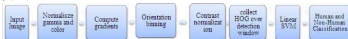
Figure 2: An overview of our feature extraction and object detection chain. The detector window is tiled with a grid of overlapping blocks in which Histogram of Oriented Gradient feature vectors are extracted. The combined vectors are fed to a linear SVM for object/non-object classification. The detection window is scanned across the image at all positions and scales, and conventional non-maximum suppression is run on the output pyramid to detect object instances, but this paper concentrates on the feature extraction process.
