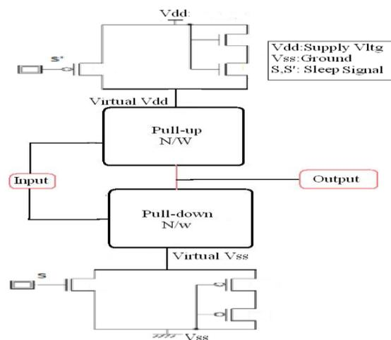
Fig6: Dual Stack Technique
