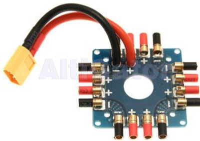
fig5. Power Distribution Board
