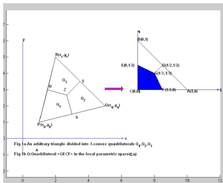
Proof: We shall now refer to Fig.1a, 1b and consider the following linear transformation between  $(x, y)$  and  $(u, v)$  spaces.
