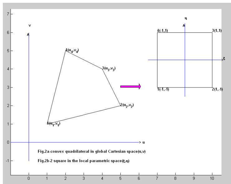
Let us consider an arbitrary four noded linear convex quadrilateral element in the global Cartesian space  $(u, v)$  as shown in Fig.2a which is mapped into a 2-square in the local parametric space  $(\xi, \eta)$  as shown in Fig.2b. The necessary bilinear transformation is given by
