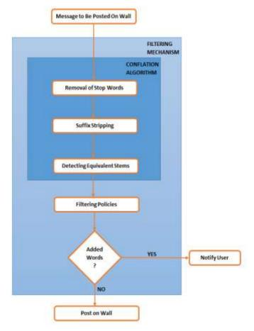
When the message is been posted the **Filtering** Wall mechanism comes into picture it works in following manner. First the input string is passed through **Conflation Algorithm**. Conflation Algorithm performs following operations on the string:
