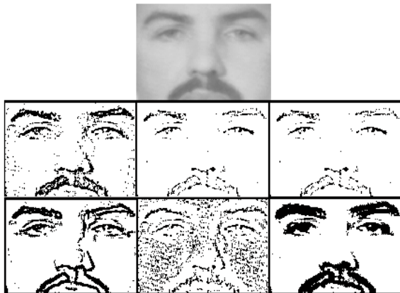
Fig 5.1:- Binarised scanned image by different techniques with local window size w=5 : (a) original image (b) LAAB at k=0.502 , (c) T.R Singh at k=0.02 , (d) Sauvola at k=0.02 . (e) Bernsen at c=0.06 (f) Niblack at k=-0.3 and (g) Proposed at k=0.9 .
