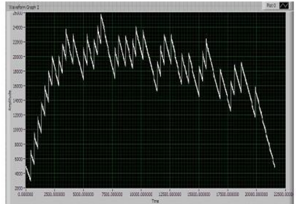
Figure 1 Acquired Waveform of Averaged Coded Stokes Trace, with 71 bit compressed multimedia information hide
