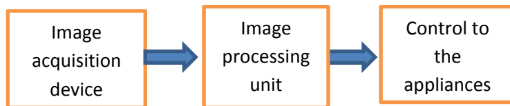
Fig2.1: block diagram of daylight sensing and processing unit
