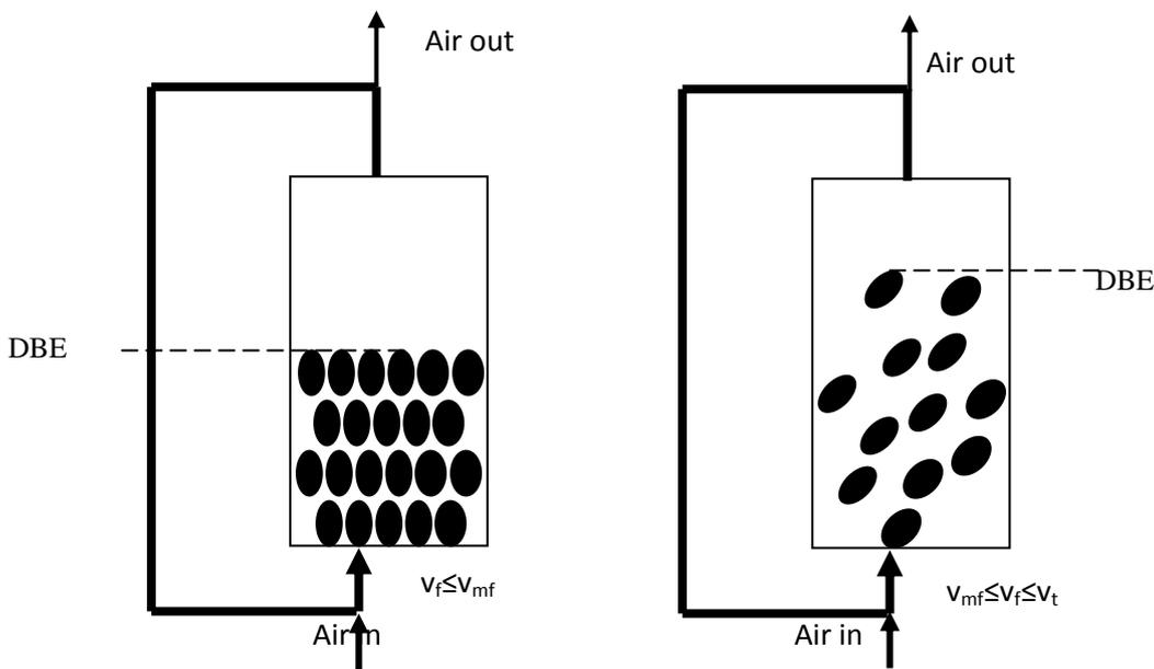
Figure 2.1: Conceptual Fluidized Reactor Containing Uniform Particles with Degree of Bed Expansion (DBE) as Related to flow velocity  $v_f$ .
