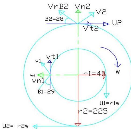
Figure 2: Velocity vector diagram of impeller wheel of the blower
