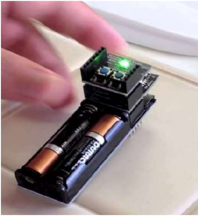
Figure 11: Battery added to beacon & signal transmission started Green LED glows indicated transmission started
