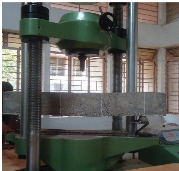
Fig 4.2 Failure of beam N-CB1
