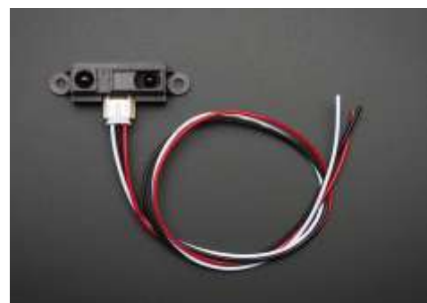
Fig 5.1.1.1 Sharp GP2Y0A21 Distance Sensor (GP2Y0A21)
