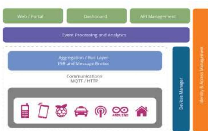
**Figure 1. Architectural Diagram for IOT**
