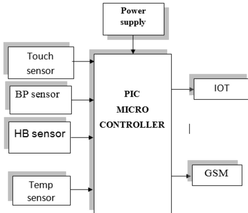
Fig.2: basic architecture of calorie and various parameter calculator
