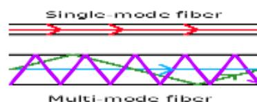
Optical fibers carry light signals down them in what are called modes. That sounds technical but it just means different ways of traveling: a mode is simply the path that a light beam follows down the fiber. One mode is to go straight down the middle of the fiber. Another is to bounce down the fiber at a shallow angle.
