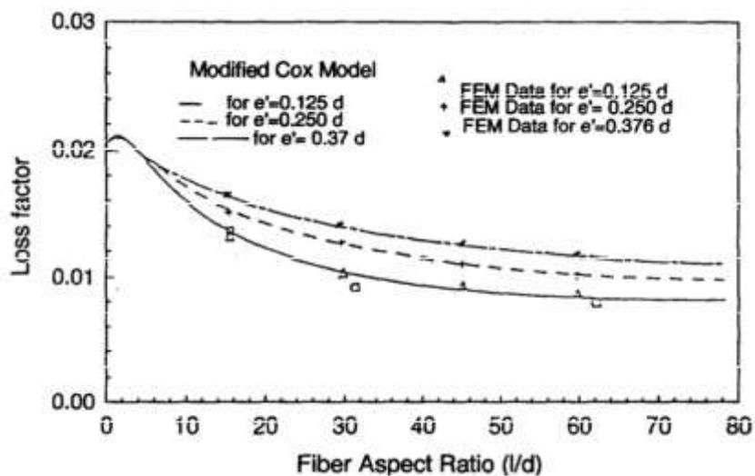
Fig-9: Plots of Loss factor vs fiber aspect ratio for Graphite Epoxy Composites using FEM data (Source: Ref-2)
