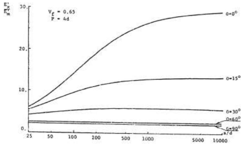
**Fig-6: Plots of  $E'_x/E'_m$  vs fiber aspect ratio using  $\theta$  as a parameter for Graphite Epoxy Composites (Source: Ref-14)**
