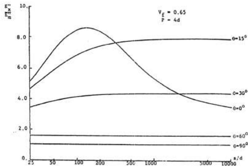
**Fig-7: Plots of  $E''_x/E''_m$  vs fiber aspect ratio using  $\theta$  as a parameter for Graphite Epoxy Composites (Source: Ref-14)**
