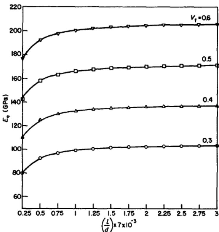
Fig-11: Variation of modulus of elasticity with fiber aspect ratio for aligned short CFRP composites (HM-S/DX21 O) for various fiber volume fractions (Source:Ref-17)
