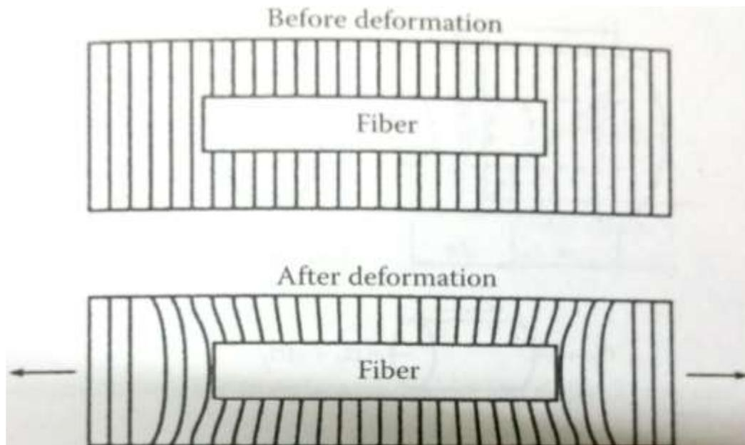
**Fig-1: Shear stress concentrations at the fiber end of discontinuous fiber reinforced composite (Source: Ref-2)**
