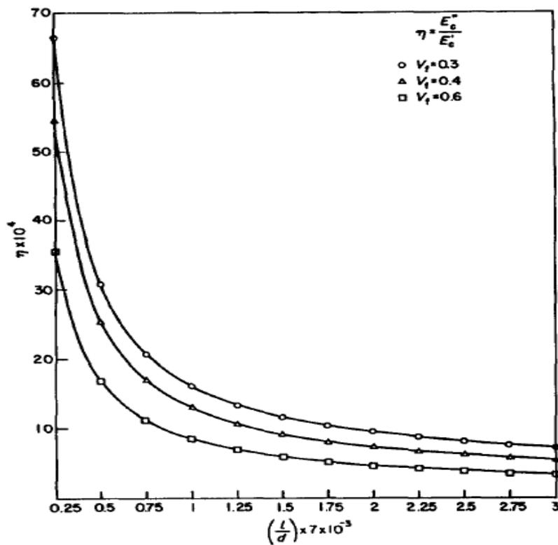
Fig-13: Variation of material loss factor with fiber aspect ratio for aligned short CFRP composites (HM-S/DX21 O) for various fiber volume fractions (Source: Ref-17)
