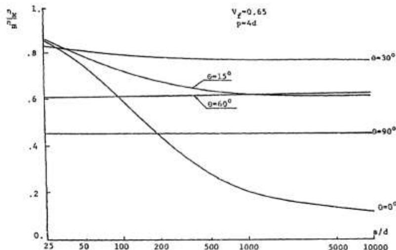
**Fig-8: Plots of  $\eta_x/\eta_m$  vs fiber aspect ratio using  $\theta$  as a parameter for Graphite Epoxy Composites (Source: Ref-14)**
