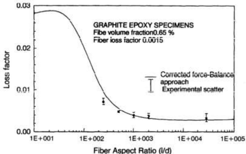
Fig-9: Plots of Loss factor vs fiber aspect ratio for Graphite Epoxy Composites (Source: Ref-2)
