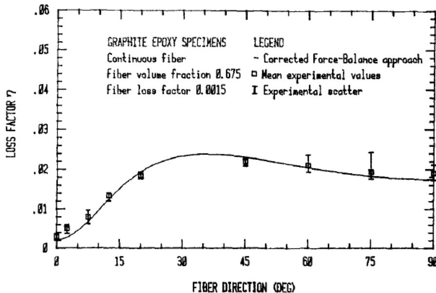
Fig-5: Predicted and experimentally obtained data for loss factor with fiber direction (Source: Ref-3)
