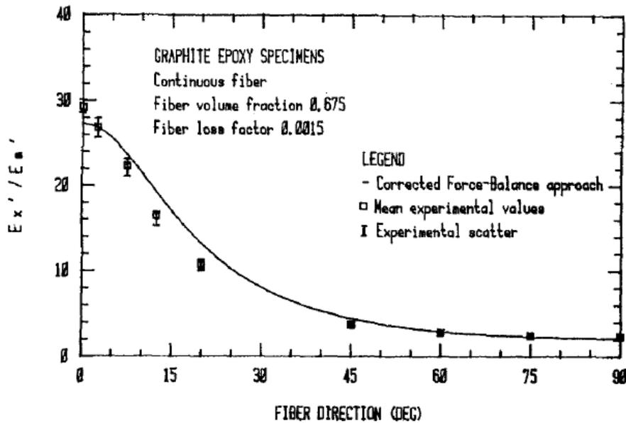
Fig-4: Predicted and experimentally obtained data for  $E'_x/E'_m$  vs fiber direction (Source: Ref-3)
