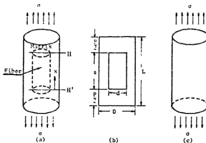
**Fig-2: Short fiber composite model (Source: Ref-16)**
