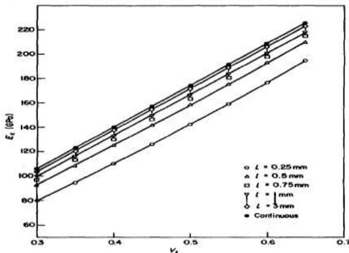
Fig-10: Variation of modulus of elasticity with fiber volume fraction for aligned short CFRP composites (HM-S/DX21 O) for various fiber lengths (Source:Ref-17)
