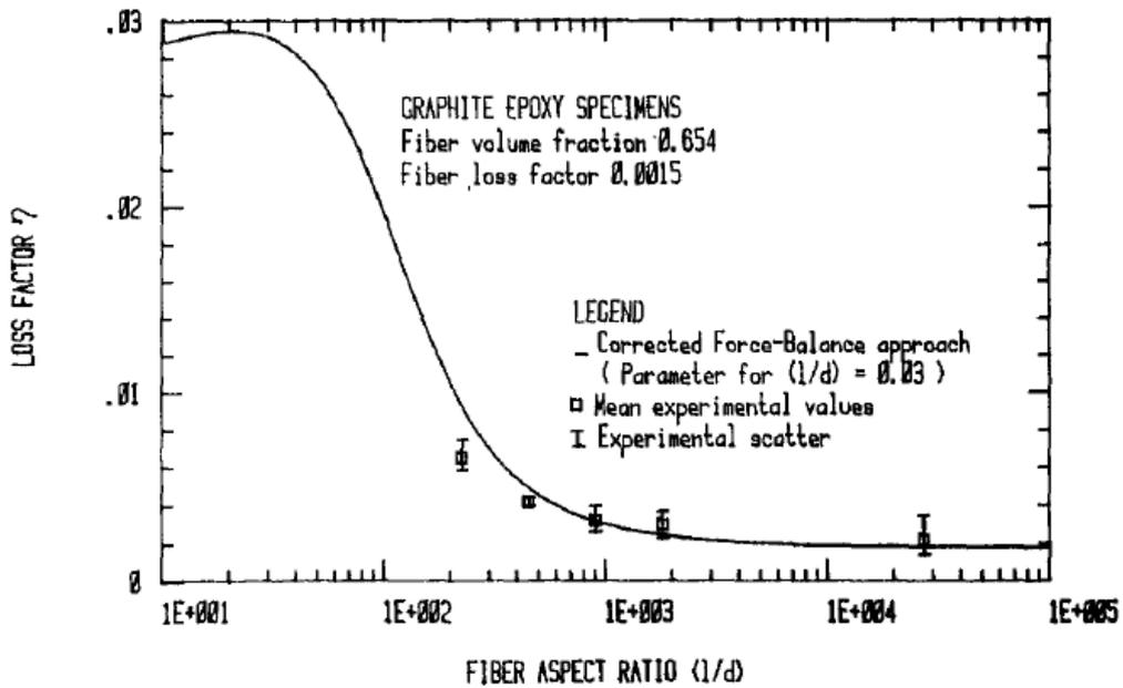
Fig-4: Predicted and experimentally obtained data for Loss factor vs fiber aspect ratio for graphite/epoxy with curve fitting (Source: Ref-3)
