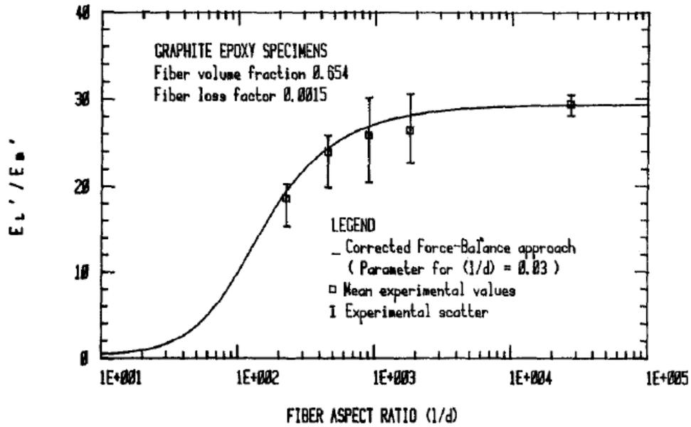
Fig-3: Predicted and experimentally obtained data for  $E_1'/E_m'$  vs fiber aspect ratio for graphite/epoxy with curve fitting (Source: Ref-3)
