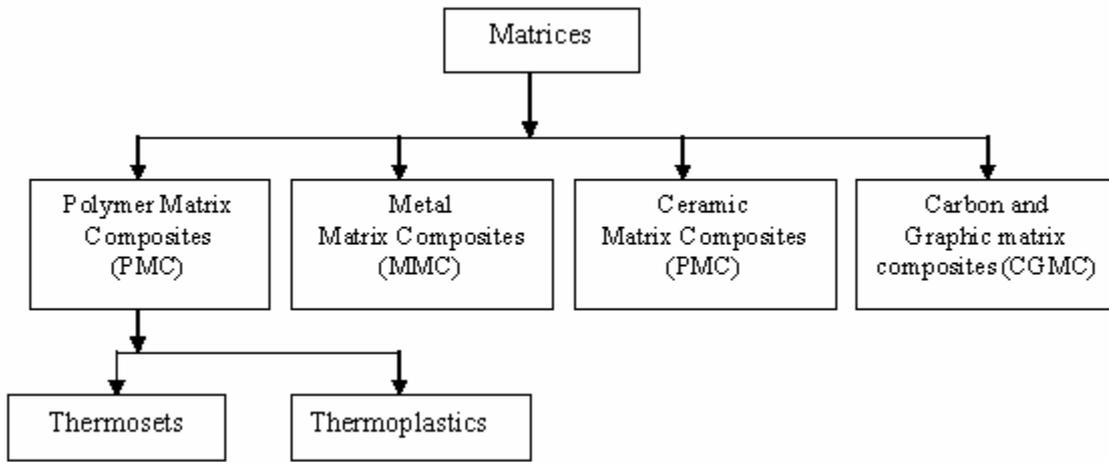
The second level of classification refers to the reinforcement form - fiber reinforced composites, laminar composites and particulate composites. Fiber Reinforced composites (FRP) can be further divided as given below.
