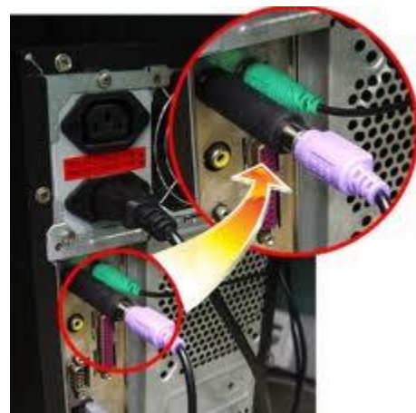
Fig.1 it shows how Hardware Keylogger is installed
