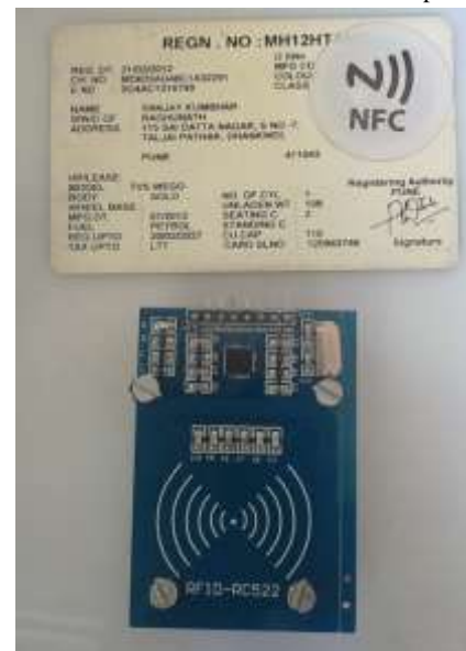
Figure 2: NFC Tag and Reader
