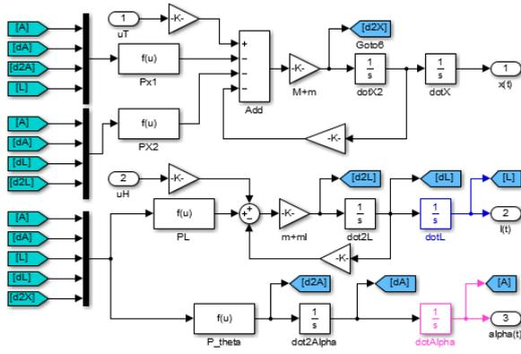
**Figure 3:** The gantry crane system modelled with SIMULINK
