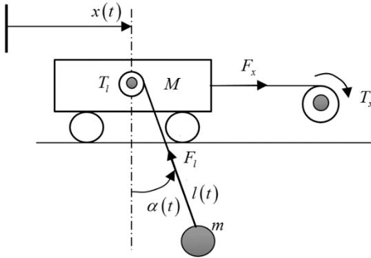
**Figure 1:** Dynamic model of gantry crane
