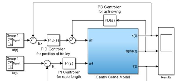
**Figure 2:** Proposed control structure for gantry crane system
