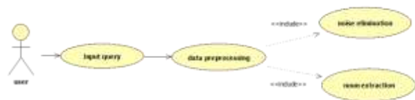
FIG 1: Use case Diagram - Input gathering and Data preprocessing
