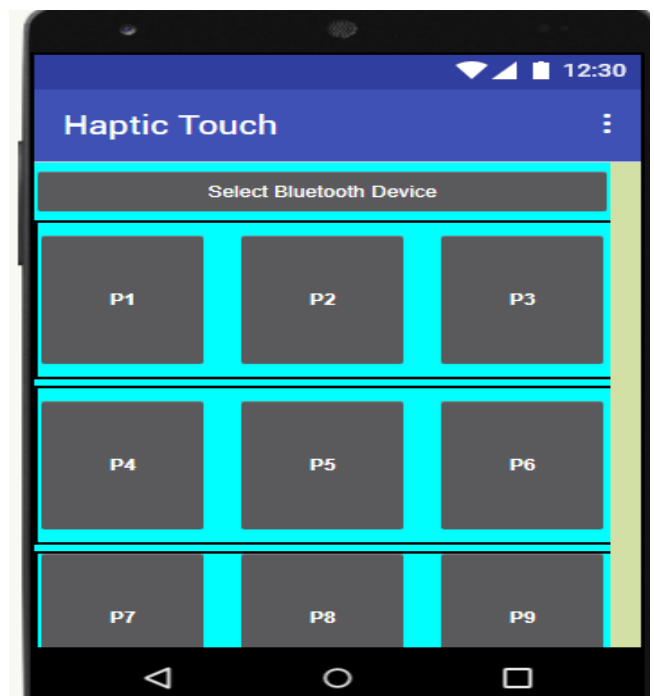
Figure 2 Displays the application's design in MIT App Inventor, featuring buttons numbered 1 to 9. Each button corresponds to a different emotion, allowing users (both transmitter and receiver) to exchange emotional signals, enhancing communication through tactile feedback.
