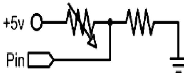
Figure 3: A circuit configuration for the NTC-Thermistor type temperature sensor (Evans, 2007)
