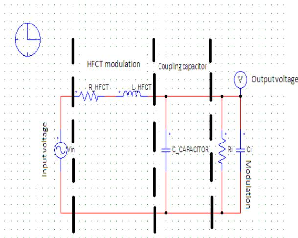
**Fig.3. simulated HFCT and c-capacitor With PSIM computer application**
