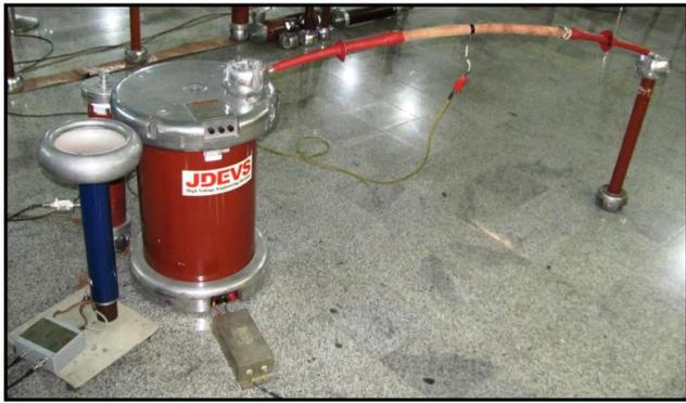
**Fig.9. Image of high voltage circuit when applying a voltage to measure partial discharge**
