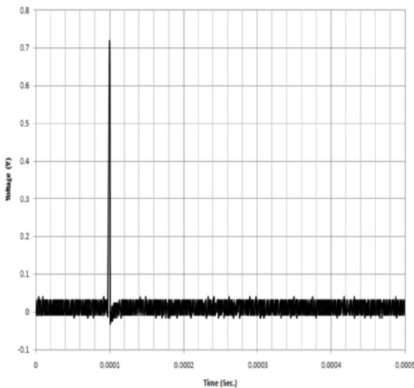
**Fig.4. A sensor response in Standard Partial Discharge**
