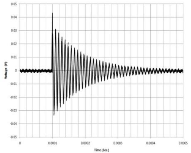
**Fig.5. A sensor response in HFCT**
