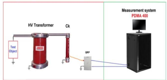
**Fig. 6. Partial discharge circuit diagram block**
