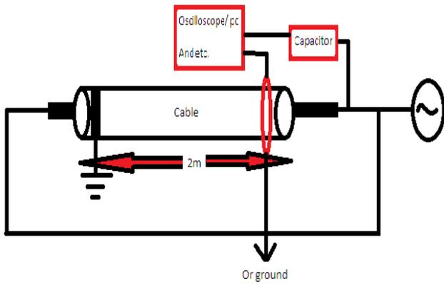
**Fig.2. Test circuit using a capacitive coupler**
