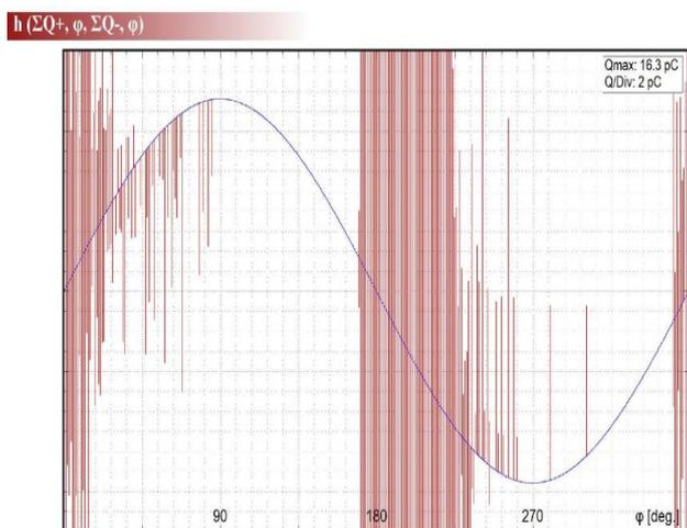
**Fig.11. Total partial discharge load diagram in terms of phase at 11.5 kV**
