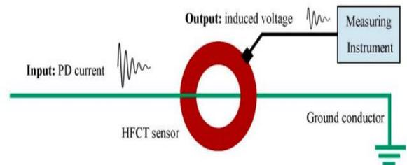
**Fig. 7. Location of the HFCT sensor in the test**
