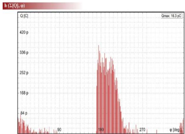
**Fig.12. Total absolute magnitude diagram of partial discharge loads by phase at 11.5 kV**
