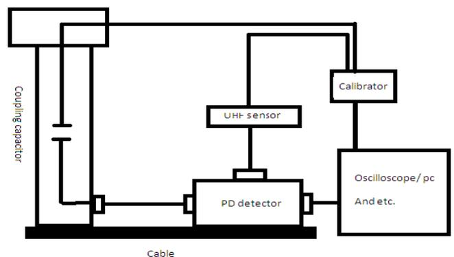
**Fig.1. schematic Placement of capacitive coupler sensor on high-pressure cable**
