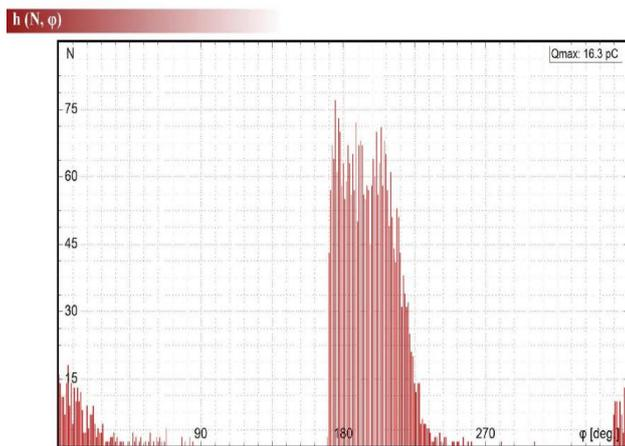
**Fig.10. The figure of the number of partial discharges per phase at a voltage of 11.5 kV**
