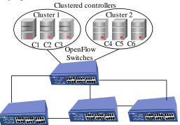
**Figure 3:** Logically centralized and physically distributed clustered controller architecture.
