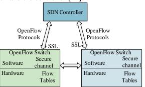
Figure 2: OpenFlow Switch architecture [20].
