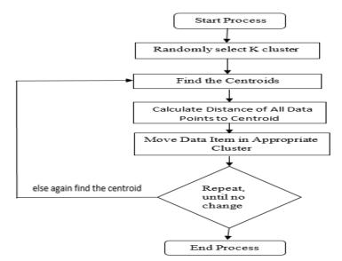
Figure 3. K-means algorithm
