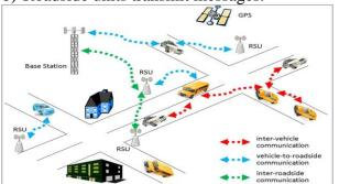
Fig 2: Communication in vehicular network [17]3. Vehicle-to-RoadsideUnit**Communication**
