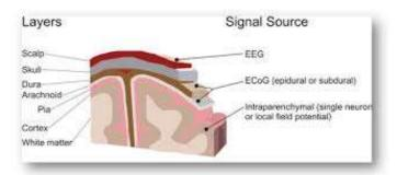
**Figure 4.2** Partially Invasive Brain Computer Interface
