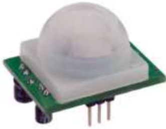
Figure: 6.4 Passive Infra Red Sensor Module
