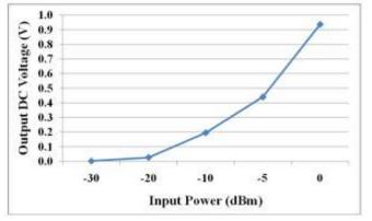
Fig.3: Output voltage and Input Power relation of schottky diode based single stage Villard voltage doubler circuit
