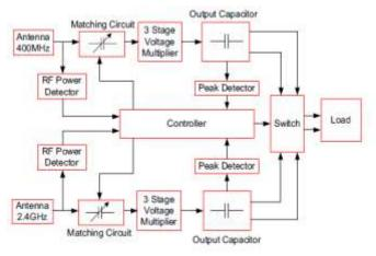
Fig.1 System Diagram of Proposed Smart RF Energy Harvester
