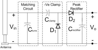
Fig.2 Single stage Voltage Doubler Circuit for converting ambient RF waves to DC
