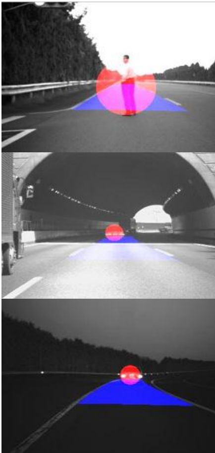
Fig. represents processing of images and detects obstacles.
