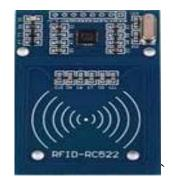
D. RFID Tags: RFID tags are passive tags which contain unique number. Whenever a passive tag comes in range of RFID scanner it send this unique number to the RFIDscanner.
